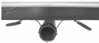
Black/Grey Tank Drain and Valves
