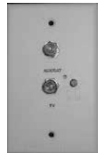
Antenna Power Supply
