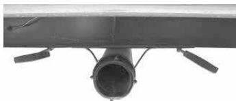
Black/Grey Tank Drain and Valves
