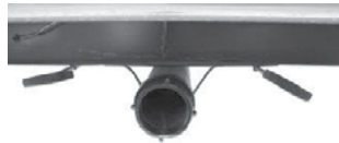
Black/Grey Tank Drain and Valves
