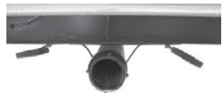
Black/Grey Tank Drain and Valves
