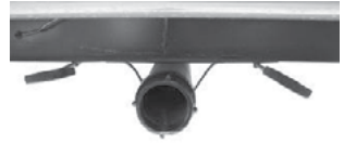
Black/Grey Tank Drain and Valves
