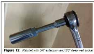
Figure 12 Ratchet with 3/8" extension and 5/8" deep well socket
