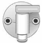
Exterior Fresh Water Drain
