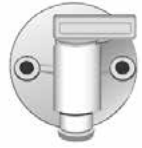
Exterior Fresh Water Drain
