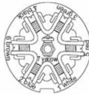
7-way trailer plug-rear view
