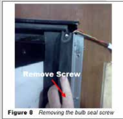
Figure 8 Removing the bulb seal screw
