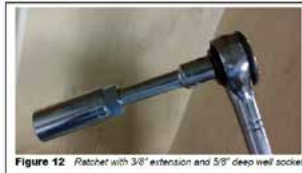
Figure 12 Ratchet with 3/8" extension and 5/8" deep well socket
