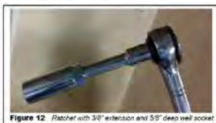
Figure 12 Ratchet with 3/8" extension and 5/8" deep well socket
