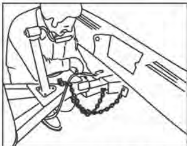
3. Repeat Step 2 with right chain. Slack for each length should be the same but not more than necessary to permit the vehicle to turn at the minimum radius.
