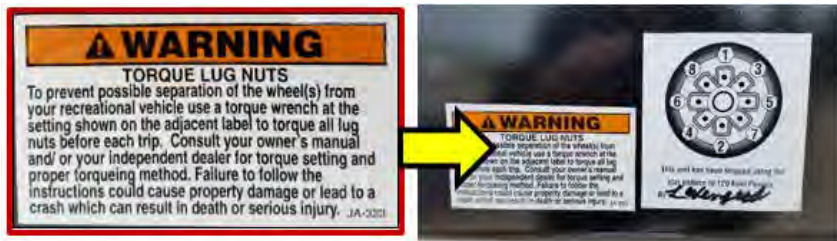
Lug nut torque pattern and warning label
