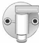
Exterior Fresh Water Drain
