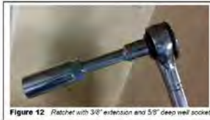
Figure 12 Ratchet with 3/8" extension and 5/8" deep well socket
